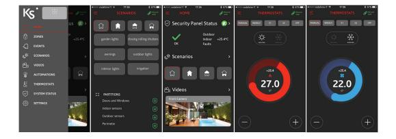
Thanks to the APP "**lares wls**", the End-User can manage entirely his System as well as the new functions of chronothermostat and Video-Verification from any mobile terminal with no need of having a Public IP Address or to configure a Router.
